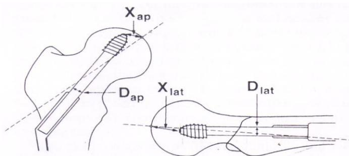
Technique for calculating the tip-apex index (TAD). For clarity, a peripherally placed screw is depicted in the anteroposterior (ap) view and a shallowly placed screw is depicted in the lateral (lat) view. ( $D_{true}$
